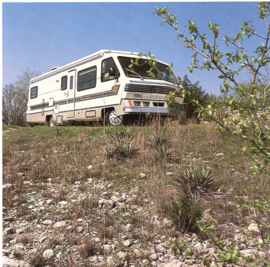
Largest EIDorado motorhome is built on a Chevrolet chassis with an extended 208-inch wheelbase and a 454-cid engine.
